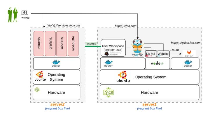
In this case, both the vagrant boxes are spawed on one server using two vagrant configuration files, namely *boxes.json* and *Vagrantfile*.
