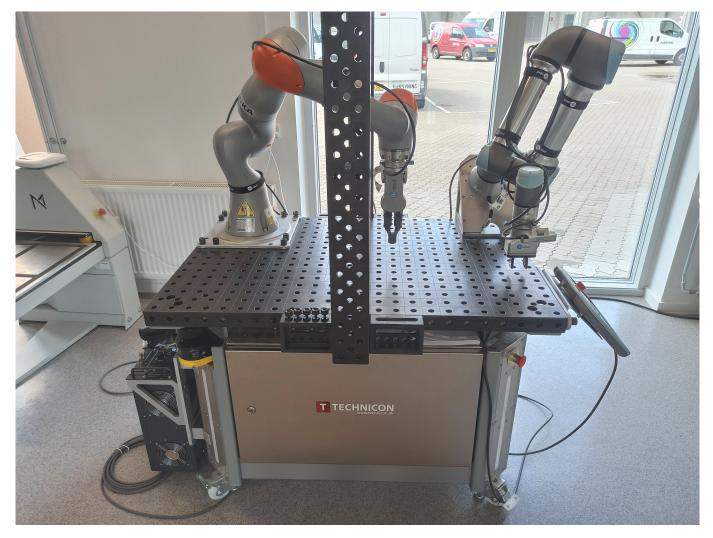
The case study focuses on the robot positioning in the discrete cartesian space of the flex-cell working space. Therefore, it is possible to send (X,Y,Z) commands to both robots, which refer to the target hole and height they want should move to.
