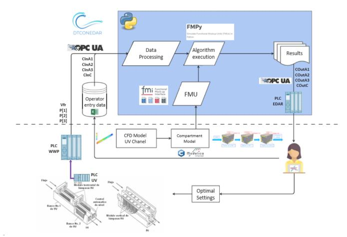
The physical twin of the waste water plant is composed of an ultraviolet channel controlled by a PLC that controls the power of the UV lamps needed to kill all the pathogens of the flow. The channel has 3 groups of UV lamps, therefore the real channel (and is mathematical model) is subdivided into 7 zones: 4 correspond to zones without UV lamps (2 for the entrance and exit of the channel + 2 zones between UV lamps) and the 3 reamaining for the UV lamps.
