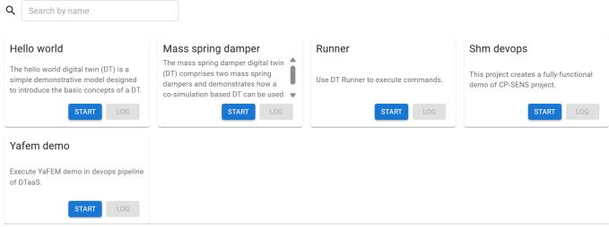
The execute tabs shows the possibility of executing multiple digital twins. Once an execution of digital twin is complete, you can see the execution log as well.
