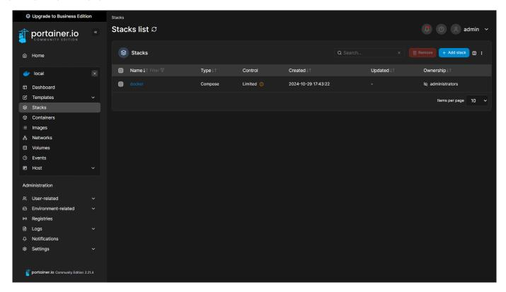
Portainer Stacks are equivalent to using docker compose commands to manage containers.
