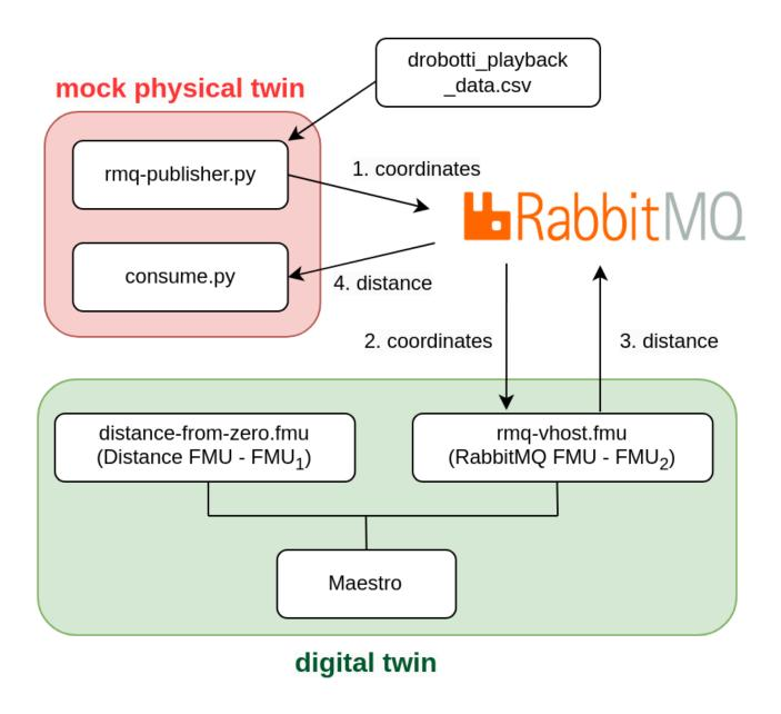
The rmq-publisher.py reads the recorded (x,y) physical coordinates of mobile robot. The recorded values are stored in a data file. These (x,y) values are published to RabbitMQ Broker. The published (x,y) values are consumed by the digital twin.
