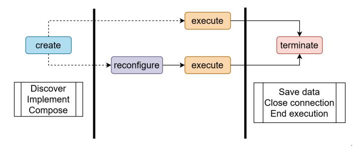
There are dedicated tabs for Create, Manage and Execute stages. The selection of DT assets for Create stage happens via Library preview page. The Manage tab fulfills reconfigure feature. The Execute and Terminate are managed on the Execute tab.
