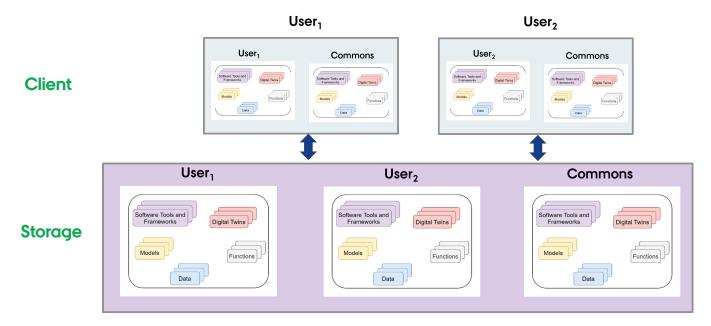
There is a skeleton file structure in DTaaS codebase. You can copy and create file system for your users. Remember to name the directory containing the file structure as files and place it in the directory from which the <code>compose.lib.yml</code> will be run.
