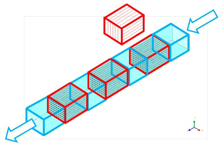
The digital twin is a reduced model (developed in C) that solves physical conservation laws (mass, energy and momentum), but simplifies details (geometry, mainly) to ensure real-time calculations and accurate results. The results are compared to the ones obtained by the CFD. C solver developed is used by the OpenModelica model. OpenModelica converts it into the FMI standard, to be integrated in the OPC UA Client (client-opcua.py).
