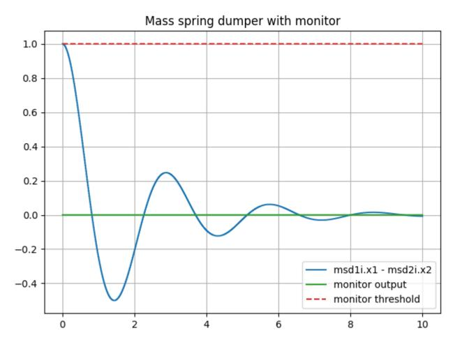
In the plot, three color-coded indicators are used to represent different values. The blue line shows the distance between the two masses, while the green indicates the monitor's verdict. A red dashed line serves as a reference point, marking the distance checked by the monitor. Since the distance of the masses is always below the threshold, the output of the monitor is fixed to unknown (0).
