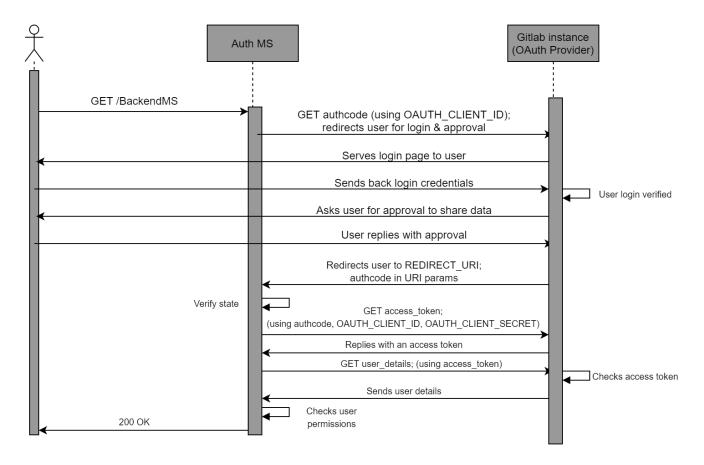
The requests made by the Auth MS to the OAuth2 provider are abbreviated. A detailed explanation of the workflow for DTaaS specifically can be found in the AuthMS implementation docs
