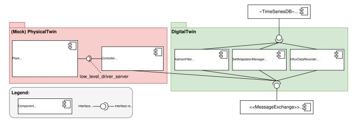
This diagrams shows the main components and the interfaces they use to communicate. All components communicate via the RabbitMQ message exchange, and the data is stored in a time series database. The RabbitMQ and InfluxDB are platform services hosted by the DTaaS.
