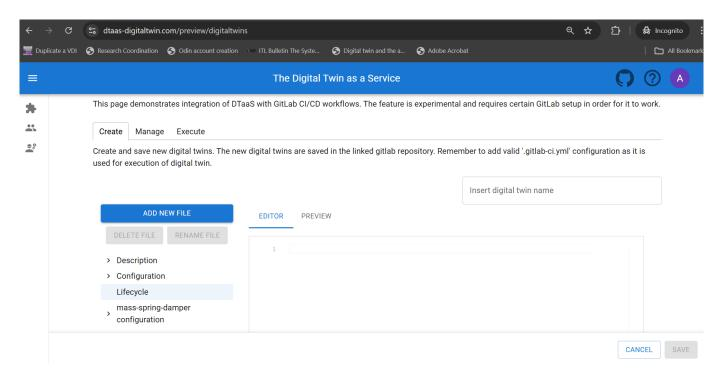
The left-side menu shows the possibility of creating necessary structure and elements for a new DT. Each reusable asset selected for this new DT' appears on the left menu. Its configuration can be updated as well.
