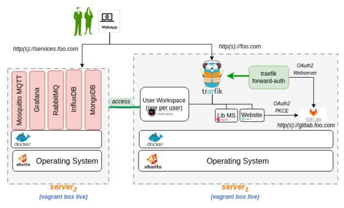
In this case, both the vagrant boxes are spawed on one server using two vagrant configuration files, namely boxes.json and Vagrantfile.
