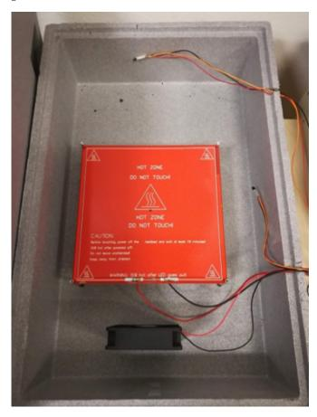
The overall purpose of the system is to reach a certain temperature within a box and keep the temperature regardless of content. An overview of the system can be seen below:
