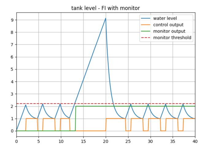
In the plot, four color-coded indicators are used to represent different values. The blue line shows the water tank level, while orange represents the control output and green indicates the monitor's verdict. A red dashed line serves as a reference point, marking the level checked by the monitor. As the water level exceeds this threshold, the monitor's verdict changes from unknown (0) to false (2).
