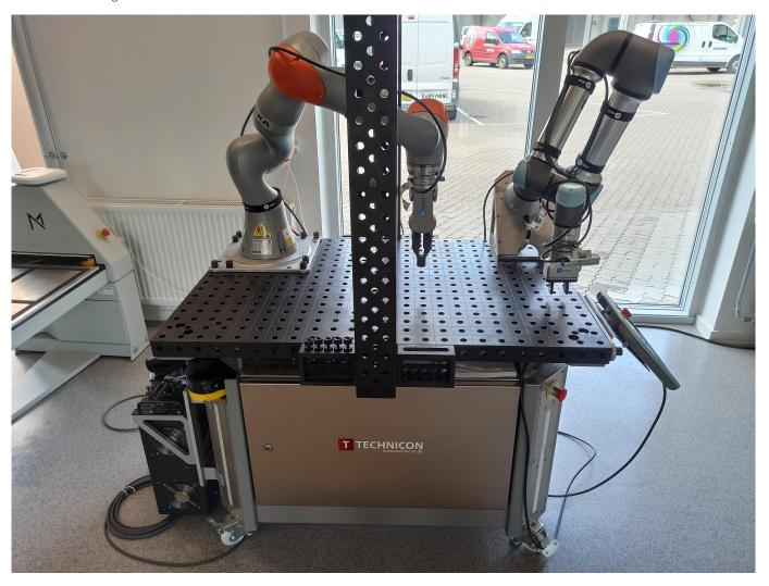
The case study focuses on the robot positioning in the discrete cartesian space of the flex-cell working space. Therefore, it is possible to send (X,Y,Z) commands to both robots, which refer to the target hole and height they want should move to.
