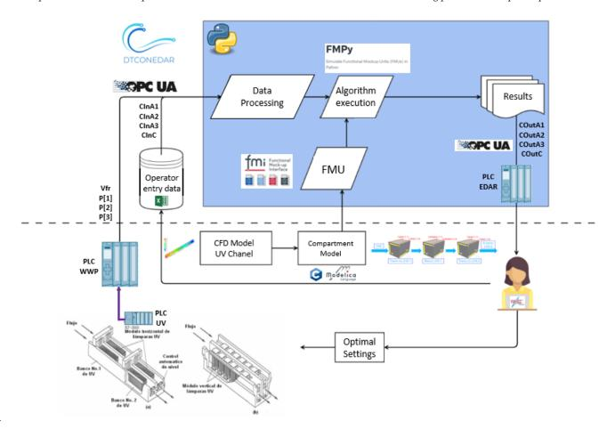
The physical twin of the waste water plant is composed of an ultraviolet channel controlled by a PLC that controls the power of the UV lamps needed to kill all the pathogens of the flow. The channel has 3 groups of UV lamps, therefore the real channel (and is mathematical model) is subdivided into 7 zones: 4 correspond to zones without UV lamps (2 for the entrance and exit of the channel + 2 zones between UV lamps) and the 3 reamaining for the UV lamps.
