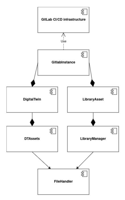
The distinction between the DigitalTwin and LibraryAsset classes was necessary to separate the full management of a DT from an asset visualized through the library. The LibraryAsset class provides a significantly reduced set of functionality compared to the DigitalTwin, focusing only on asset visualization.
