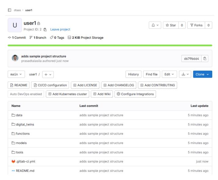
Please pay special attention to <code>.gitlab-ci.yml</code> . It must be a valid Gitlab DevOps configuration. You can also check example repo for a sample structure.
