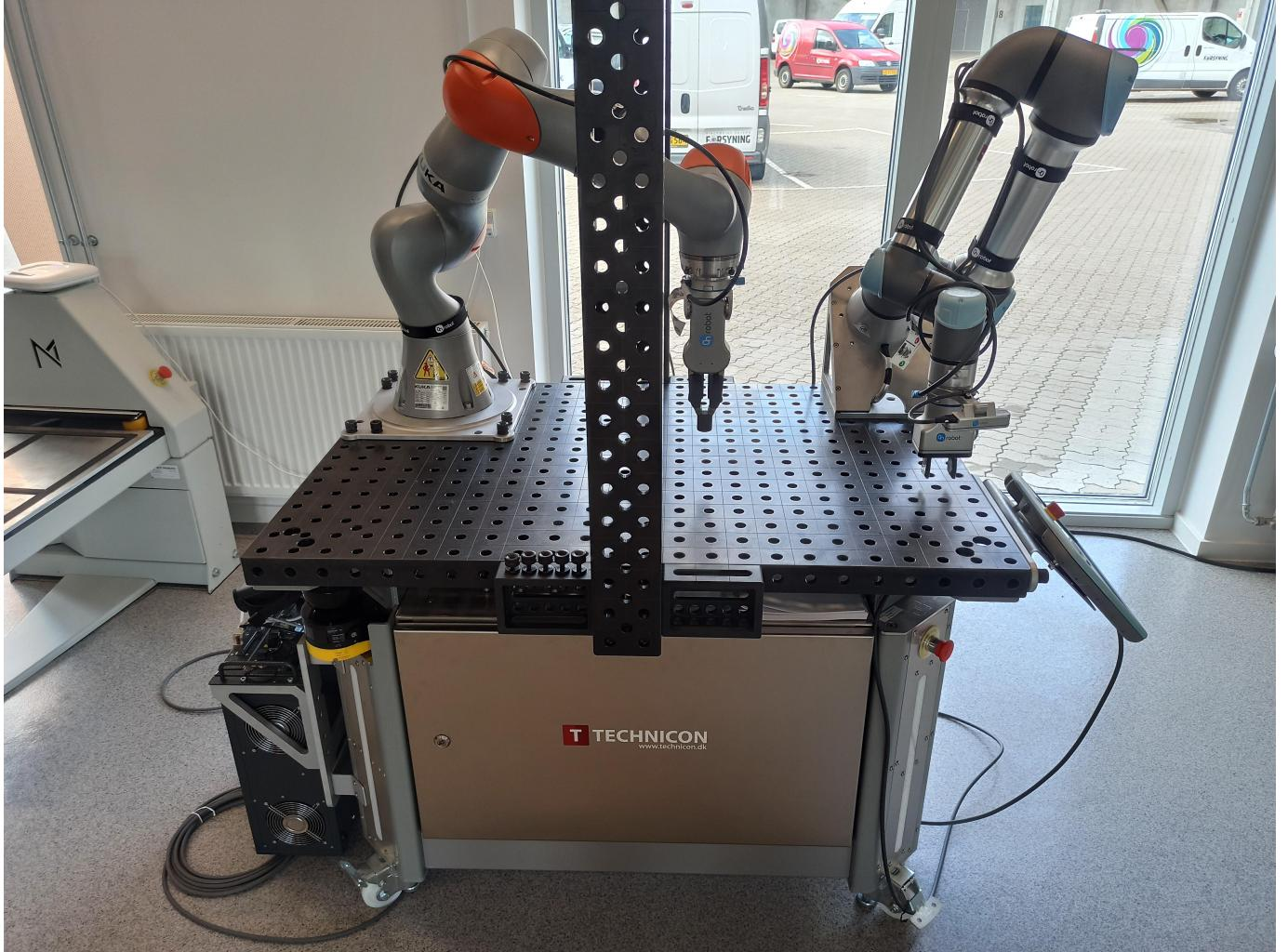
The case study focuses on the robot positioning in the discrete cartesian space of the flex-cell working space. Therefore, it is possible to send (X,Y,Z) commands to both robots, which refer to the target hole and height to which they should move.
